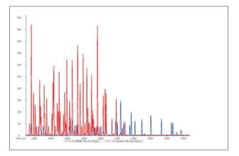
Figure 3. Overlaid one-dimensional ECD chromatograms for a PBDE standard mix (blue) and a PCB Aroclor mix (red). Numerous coelutions occur under these GC conditions.
