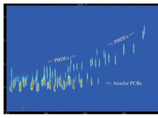
Figure 1. Contour plot showing GCxGC-ECD separation of PCBs and PBDEs. Note the separation of compounds in two dimensions with the Rtx-5 separation (and retention time) on the X-axis and the DB-17 separation occurring along the Y-axis.
