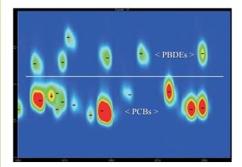
Figure 2. Zoom of Figure 1 contour plot showing distinct separation of PCBs and PBDEs in the second dimension when using GCxGC-ECD.
